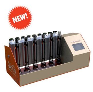
Laboratory shaker OLISLAB 6300 is designed for uniform distribution of a solid dispersed phase (flour or crushed grain) in a liquid dispersion medium (water or organic solutions) to form a homogeneous suspension by shaking according to a specific program.
